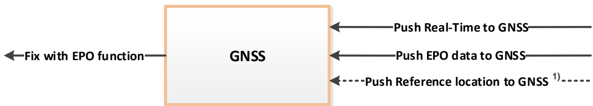
Figure 2: EPO™ Function Operation Flow
